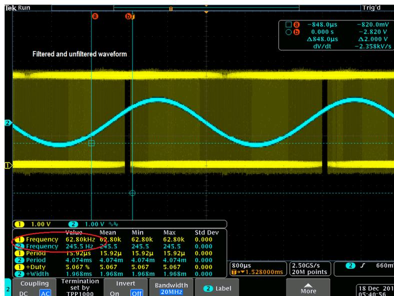
Figure 4-2. PWM Output and Sine Wave – Zoomed View
