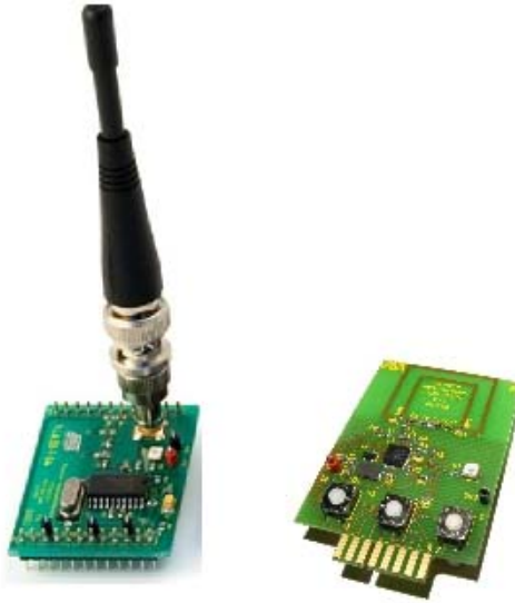
Figure 1. Secure Rolling Code Development Tools (STK512)
