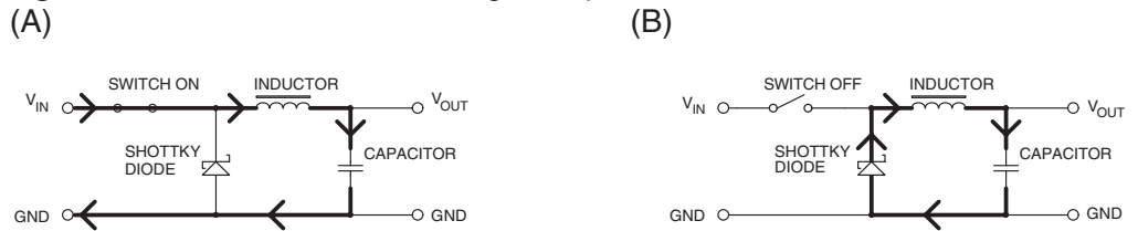
Figure 3-2. Buck Converter Switching Principle
