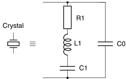
This model can be associated to the crystal manufacturers' parameters. See Table 1.
