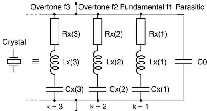
The parasitic capacitance of the crystal’s electrodes and the package are modelled by the capacitor  $C_0$ . Together with the motional inductance  $Lx(k)$  this capacitor forms resonant circuits that also produce parallel resonant frequencies  $fp(k)$ . They cannot be used for oscillation with the type of oscillators presented here.
