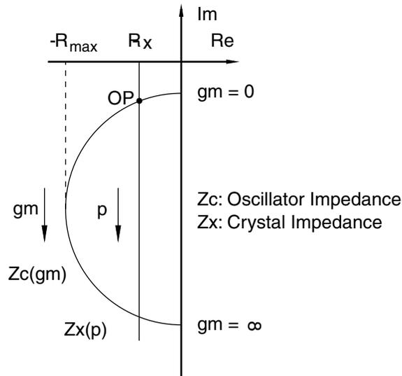
The complex plane representations of  $Z_c$  as a function of  $gm$  and of the crystal impedance  $Z_x$  as a function of its frequency pulling  $P$  are shown in Figure 4. The formula for the real and imaginary parts of  $Z_c$  are also given. The two intersections of  $Z_c$  and  $Z_x$  are the possible operating points of the circuitry, according to the critical condition for oscillation.
