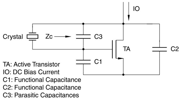
$C_3$  is a parasitic capacitance that includes package capacitance of the crystal ( $C_0$ ), board capacitance and internal parasitic of the oscillator circuit such as the Miller
