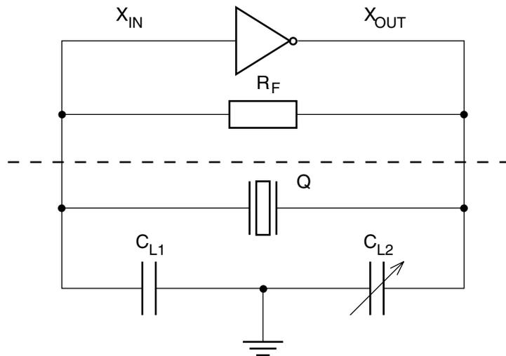
The resultant load capacitance  $C_L$  is given from  $C_{L1}$  and  $C_{L2}$  by the following formula:
