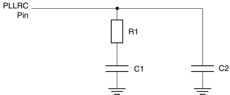
The filter's purpose is to transform the  $I_d(t)$  current issued from PFLD/CP block into a voltage  $V_{ref}(t)$ :
