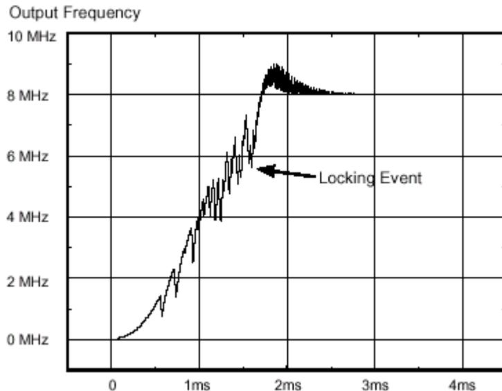
As a result of the oscillatory process as described above, during the lock period of the PLL the derived clock frequency may vary significantly with respect to the target fre-
