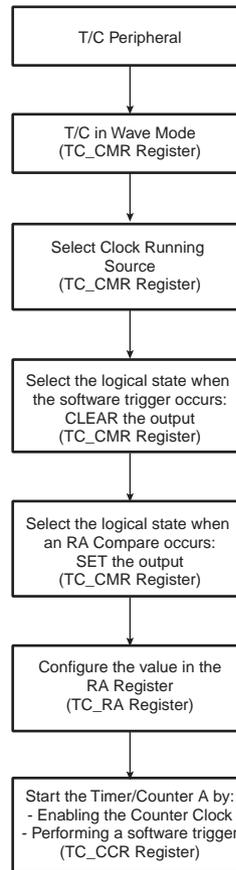
When a Timer/Counter output is used to trigger the conversion, the multiplexed I/O controller must first be disabled on the targeted pin.
