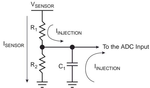
The value of the capacitor must be sufficient to transfer the necessary charges and show a voltage variation less than a quantum of conversion. Inversely,  $C_1$  must not be overvalued: Out of the track period (between two consecutive measurement or a measurement sequence), the full load must be reach through the equivalent impedance equal to:
