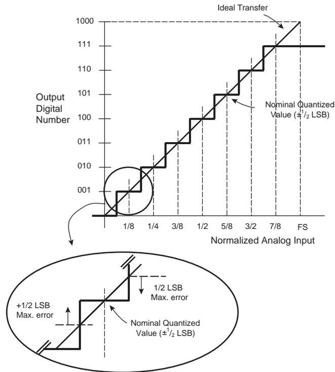
An n-bit converter is able to discriminate  $2^n$  different states. We say that the resolution is equal to n bits. The relative accuracy is given by:
