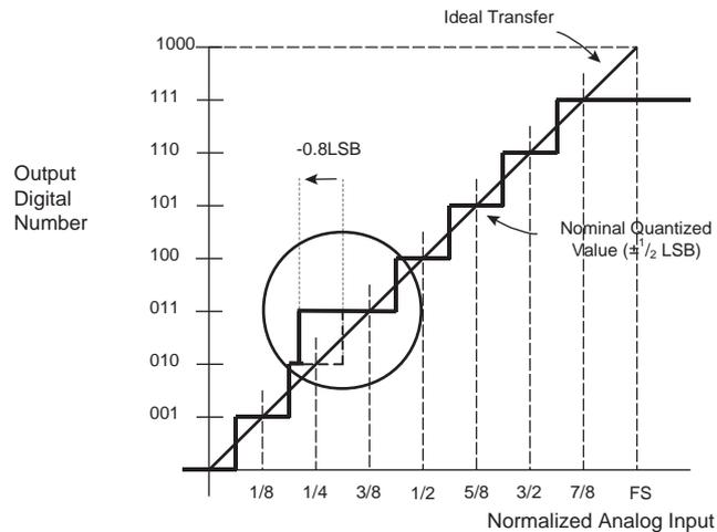
Figure 3 illustrates a DNL error between the code 0b100 and 0b110. The DNL error is equal to the real gap value between the code 0b100 and the next minus the 1 LSB theoretically expected: 2 LSB - 1 LSB = +1 LSB of DNL error in this case.
