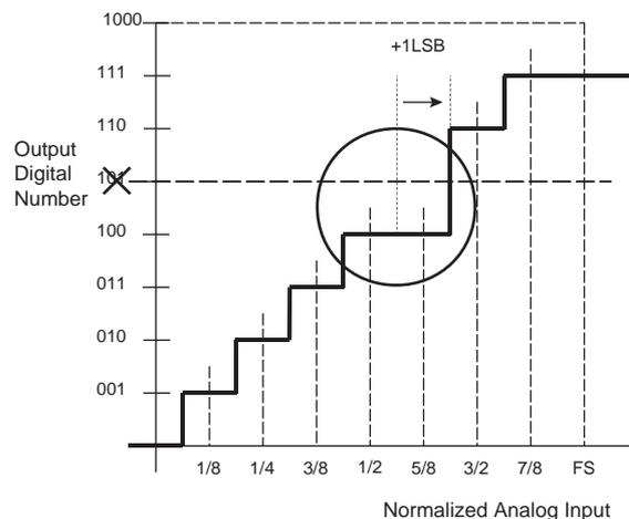
In this last example, the DNL error is greater than 1 LSB, the code width vanishes entirely and the ADC has at least one missing code.
