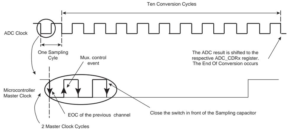
Figure 11 also shows that, in order to avoid a deterioration in sampling time due to both master clock cycles, it is important that the ADC frequency is lower than the master clock frequency. The calculation of input impedance takes this constraint into account.
