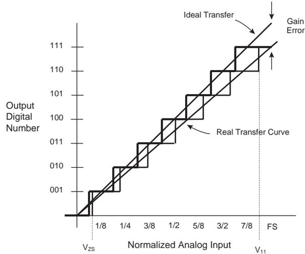
To determine the gain error of an ADC, measure the final transition voltage and subtract the first transition voltage. Since this interval is ideally equal to  $(V_{FS} - 2 \text{ LSB})$ , the deviation of the difference of the measured values from the value of  $(V_{FS} - 2 \text{ LSB})$  is the full-scale gain error. The gain error can be expressed in LSBs. The gain error of Figure 6 may be determined by the following equation:
