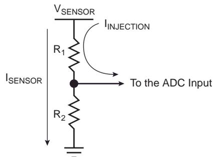
In order to decrease the continuous  $I_{SENSOR}$  leakage through  $R_1$  and  $R_2$ , the user selects the higher bridge value without exceeding the previously given  $Z_{MAX}$  so that  $I_{INJECTION}$  is sufficient.
