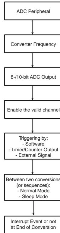
**Detailed Sampling Period** The ADC peripheral can provide 8- or 10-bit output data. Note that the 8-bit mode does not decrease conversion time; in both modes, 11 ADC clock cycles are required to perform a full conversion. The major difference between the two modes is that in 8-bit mode data handling is easier when the software needs to work in byte mode.
