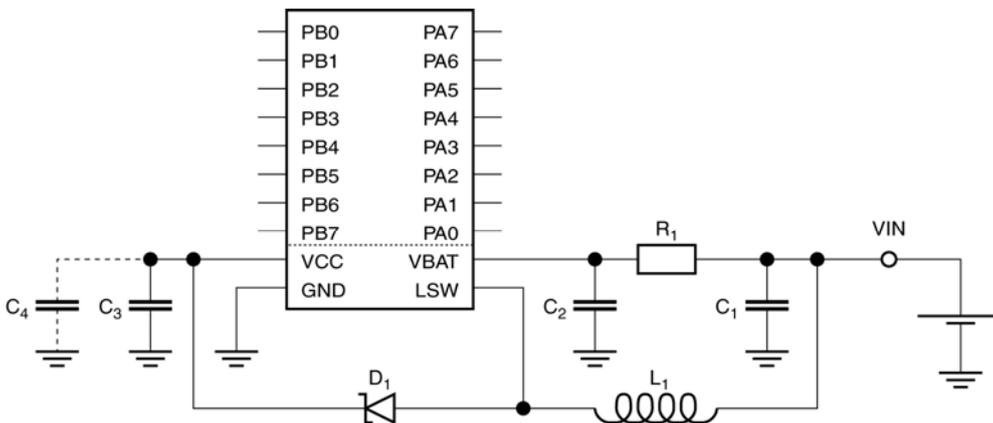
The boost converter continuously switches between storing energy in and draining energy from the external inductor. During the charge phase the current in the inductor ramps up at a rate determined by the converter input voltage. During the discharge phase energy stored in the inductor is released to the load and the current in the inductor ramps down at a rate determined by the difference between the input and output voltages.
