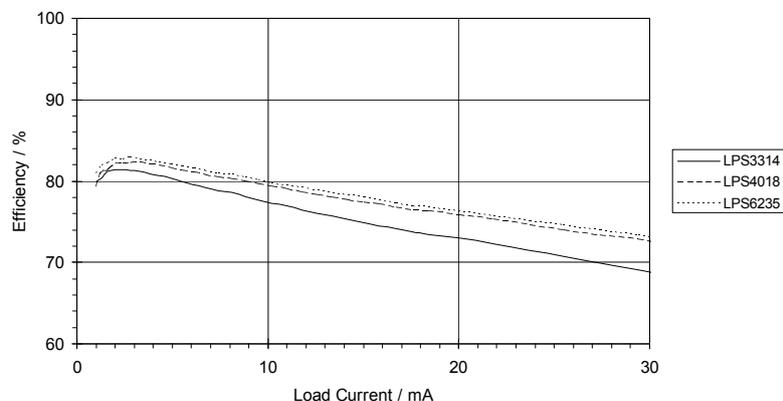
Core losses are device specific and are given by coil manufacturers. The lower the core loss the better the efficiency of the boost regulator.
