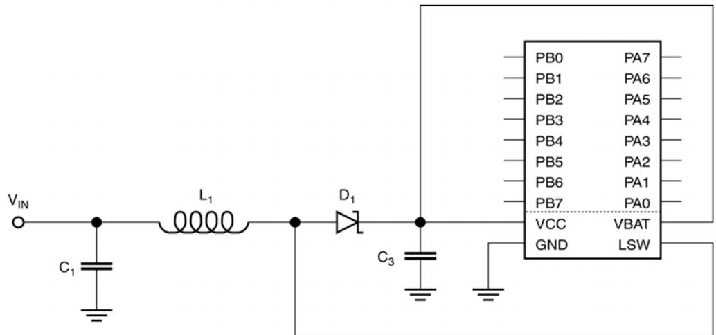
When battery is drained the boost converter input voltage drops and the efficiency of the converter decreases. This means that at lower input voltages more input current is required to generate the same load current. It also means that at lower voltages the maximum load current the boost converter can provide decreases. This is illustrated in Table 6-1 below, where  $I_{LOAD}$  is the maximum current the boost converter can provide while still maintaining regulation.
