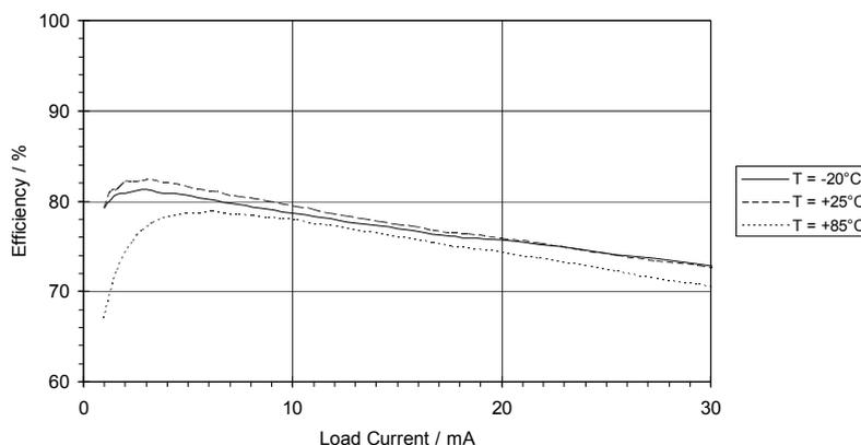
The temperature dependency of  $V_F$  and  $I_R$  are particular to the make and model of diode used. Figure 2-3 below illustrates how booster efficiency at high temperatures is affected by the type of diode used. Component values (excluding the diodes) are those listed in Table 2-1.
