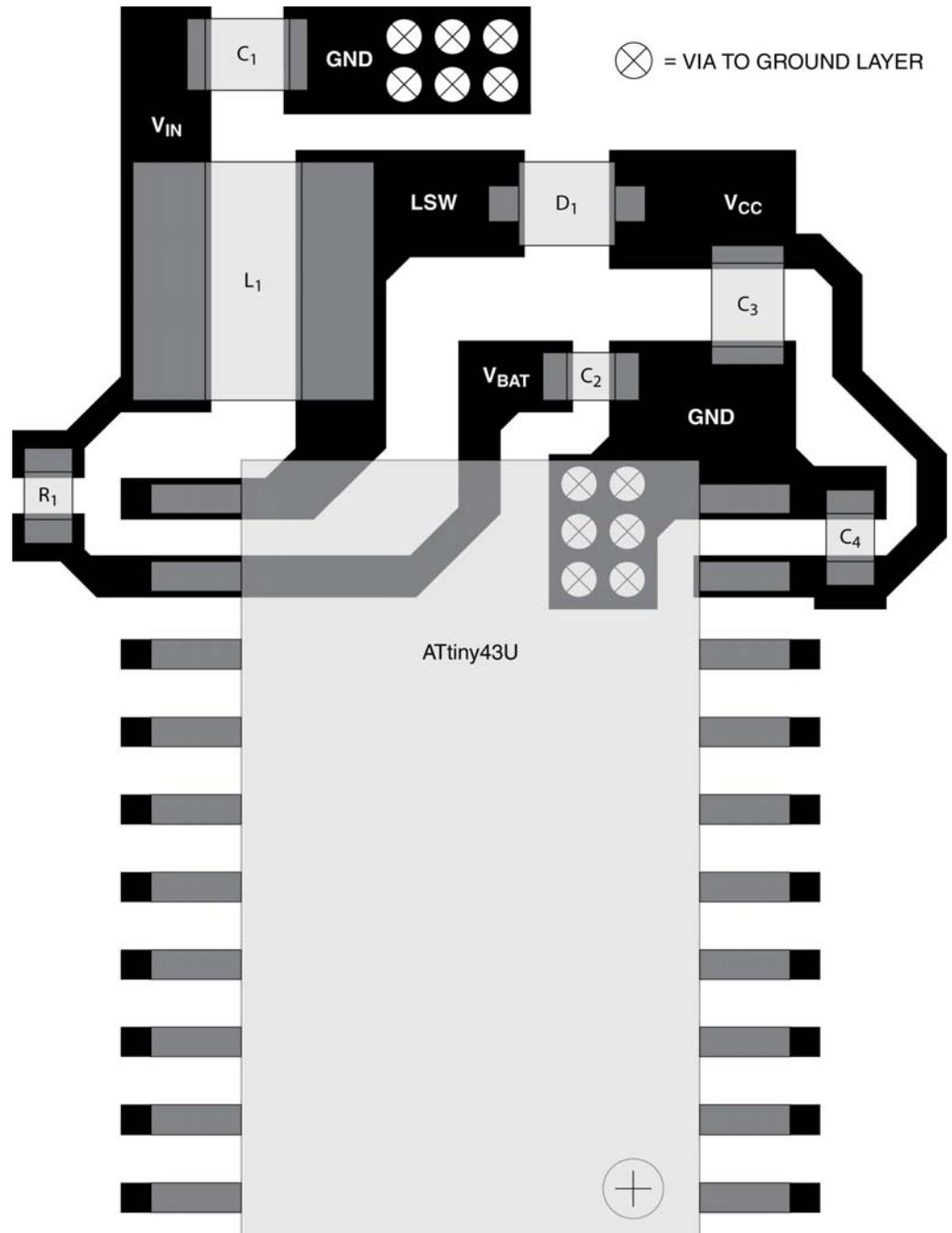
In addition to the top layer, it is also recommended to include a separate ground layer and bolt the ground areas of the top layer to the ground layer firmly by several vias. Ground fillings in the top layer are to be avoided since they are prone to pick up noise.
