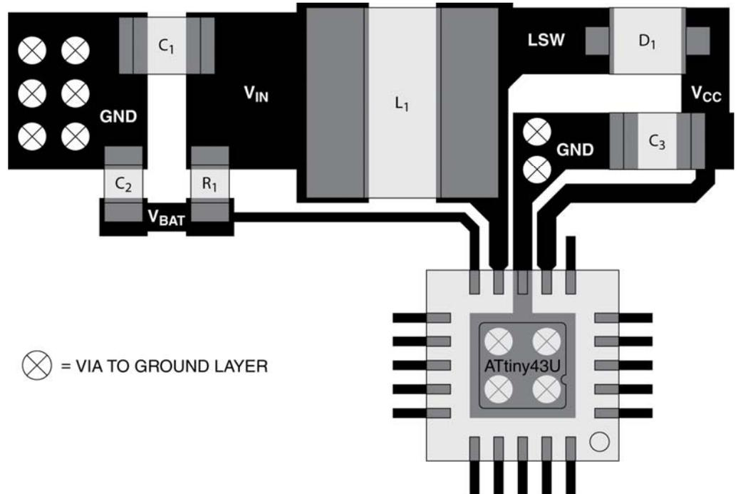
In addition to the top layer, it is also recommended to include a separate ground layer and bolt the ground areas of the top layer to the ground layer firmly by several vias. The exposed die pad of the MLF package should be connected to the ground layer through via matrices. Ground fillings in the top layer are to be avoided since they are prone to pick up noise.
