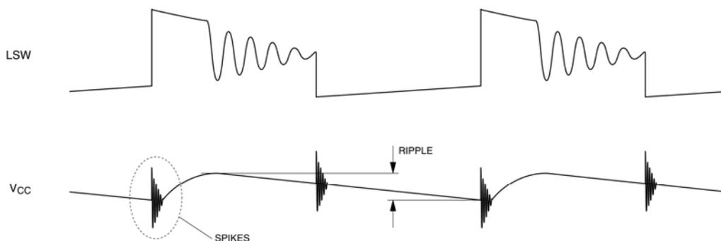
Supply voltage ripple and spikes do not affect the operation of the boost regulator but may be undesired in some applications.
