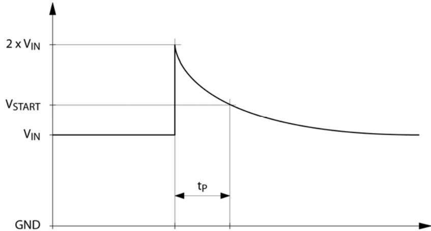
For the low voltage start circuitry to be successful the voltage at  $V_{BAT}$  needs to remain above the start level  $V_{START}$  sufficiently long. The time required,  $t_p$ , depends on the battery voltage and the peak amplitude. Typical values are summarized in Table 5-1 below. The values given assume a worst-case start voltage of 1.35V. Actual values may be lower.
