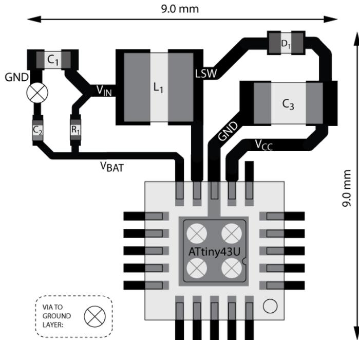
The spacing between components in this layout is 1 mm in minimum. Depending on the selected component mounting process the spacing can be adjusted accordingly. The line widths are 0.3 mm in the power path (V<sub>IN</sub>, L<sub>SW</sub>, V<sub>CC</sub> and GND wires). The line thickness should be selected so that the wires can sustain RMS currents of up to 250 mA.
