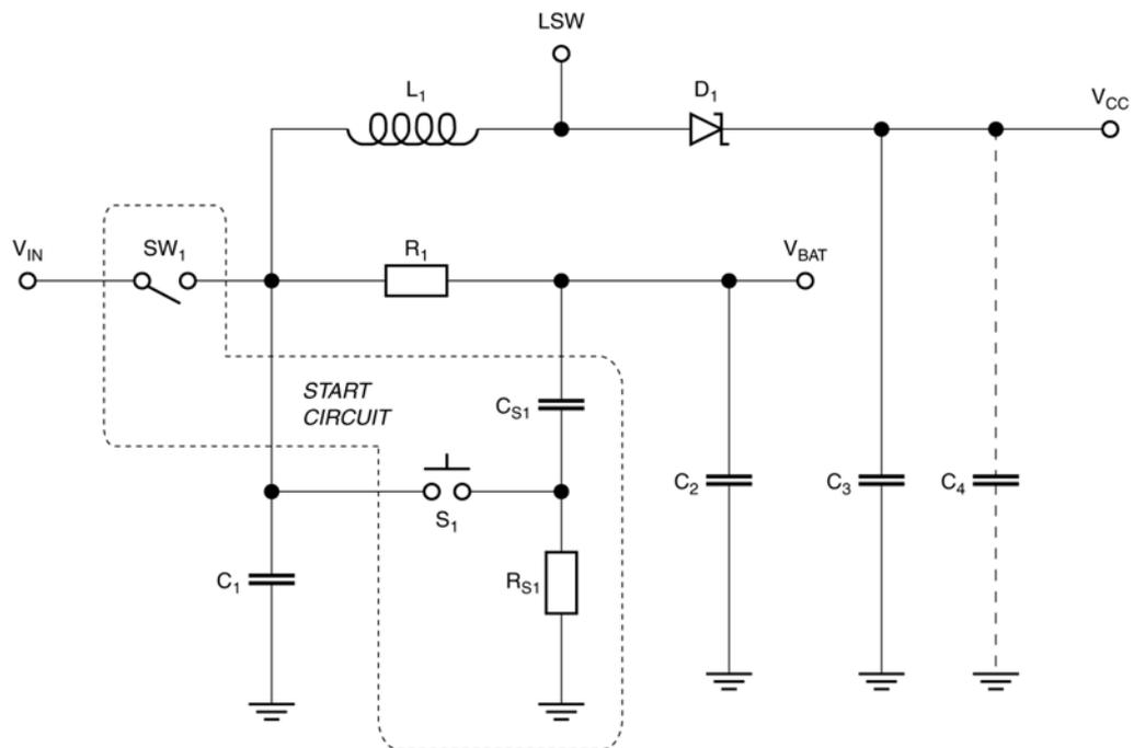
When button,  $S_1$ , is pushed the supply voltage is momentarily raised to a level above start voltage, allowing the boost converter to start.
