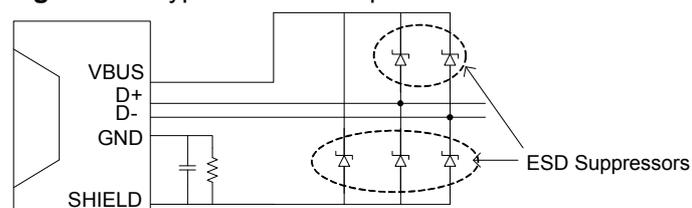
The ESD suppressors can be independent, discrete protection devices or specific, integrated USB protections.
