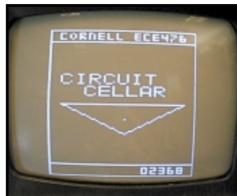
Photo 1: The "Cornell ECE476" message and time in the lower right corner are computed by the program. The "Circuit Cellar," triangle, and dot are the result of commands issued to the Mega163 from HyperTerminal. The commands are: t0530CIRCUIT (text starting at x = 05, y = 30); t1538CELLAR; L055058501 (line x1 = 05, y1 = 50, x2 = 58, y2 = 50, color = 1); L055032701; L585032701; and p32601 (point x = 32, y = 60, color = 1).
