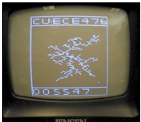
Photo 2: This DLA program example takes 5547 s to compute. You can see the current free particle as a blur in the lower right corner of the screen.
