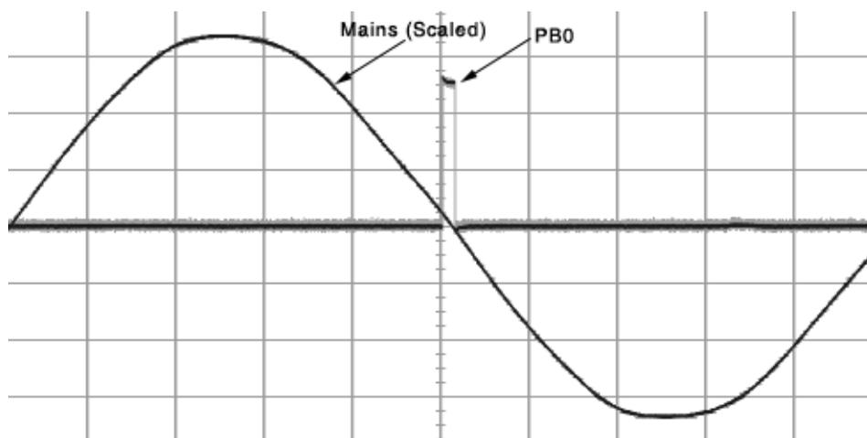
In a real application the disabling of external interrupt 0 before returning from the interrupt routine will make a single detection. To detect a new zero crossing, simply enable the falling edge interrupt again in the main program.
