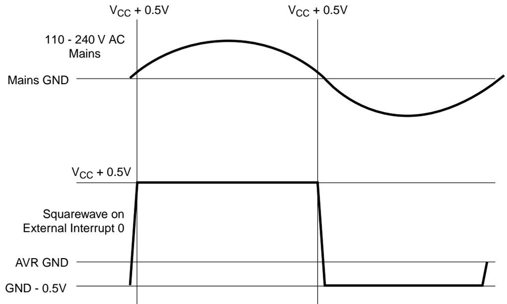
**Figure 3.** Oscilloscope Screenshot of Square Wave Input on External Interrupt 0-pin
