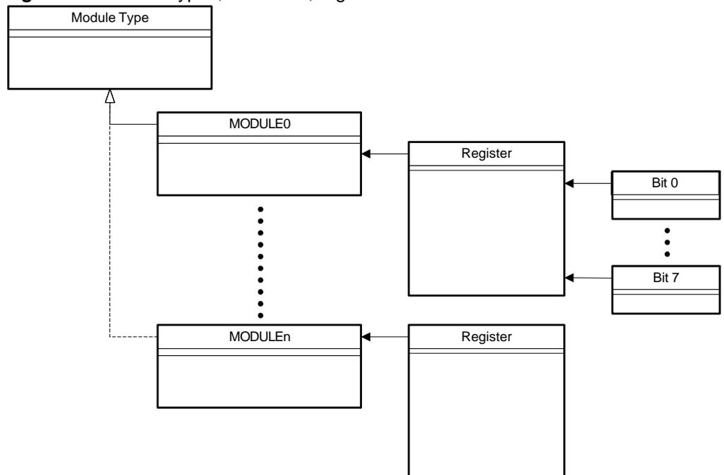
Each module has a fixed base address in the IO memory map and all registers contained in the module have fixed offset addresses relative to the module base address. This way each register will not only have an absolute address in the IO memory space, but also a relative address defined by its offset. The register offset addresses are equal for all instances of a module type, simplifying the task of writing drivers that can be used for all modules of a specific type.
