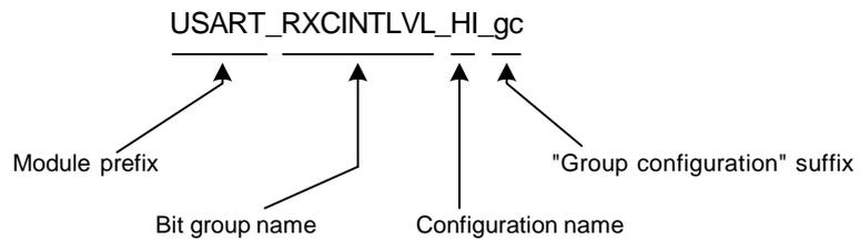
Inspecting the group configuration Figure 3-2, one can see that it is used to select a configuration for the `RXCINTLVL` bits in a USART module. This specific group configuration selects a high (HI) interrupt level.
