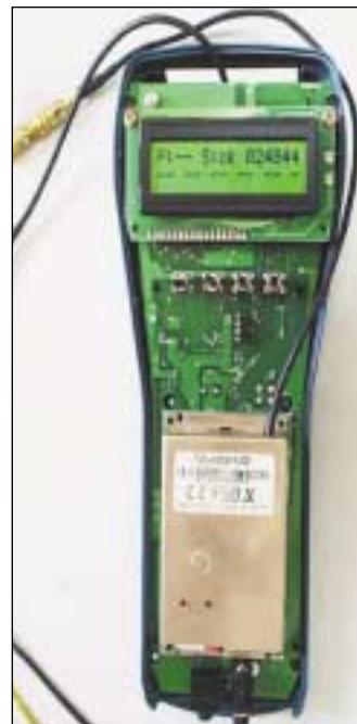
Photo 1—On the front side of the main board, you can see an LCD, four programmable keys, a GSM module, an RS-232 connector, and some other components.
